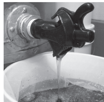
The uncapped frames are loaded into the extractor. The extractor is spun and centrifugal force extracts the honey from the frames. The honey collects in the bottom of the extractor and then is poured and strained (below) from the extractor.
