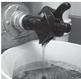
The uncapped frames are loaded into the extractor. The extractor is spun and centrifugal force extracts the honey from the frames. The honey collects in the bottom of the extractor and then is poured and strained (below) from the extractor.
