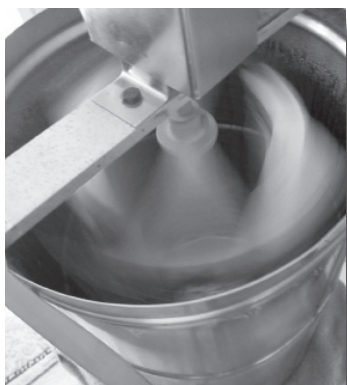
The uncapped frames are loaded into the extractor. The extractor is spun and centrifugal force extracts the honey from the frames. The honey collects in the bottom of the extractor and then is poured and strained (below) from the extractor.
